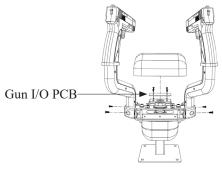
Replace the GUN I/O PCB and reassemble in reverse order
