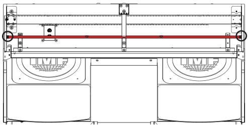
Insert the Panel Header Mid Artwork (MI-5712X-AUK) and secure using the (3) M4 highlighted fixings
