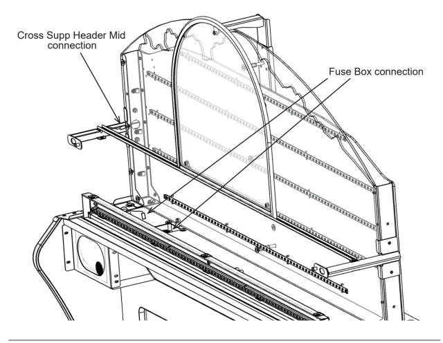
Insert the **Panel Header Front Artwork (MI-5711X-AUK)** and secure using the (2) M4 highlighted fixings
