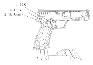
Reassemble the Controller unit following these instructions in reverse order. Check operation using the OUTPUT TEST MODE in section 9 of this Manual
