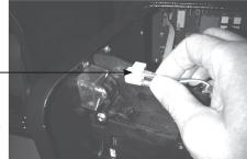
Step 3. Once the Lamp Housing has been removed, carefully hold the bulb between your fingers and pull the Lamp Housing away.
