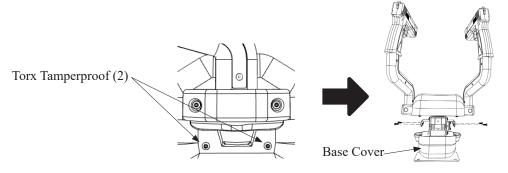
Remove the (2) machine screws which retain the cover bracket. This will enable you to gain access to the VERT Controller PCB
