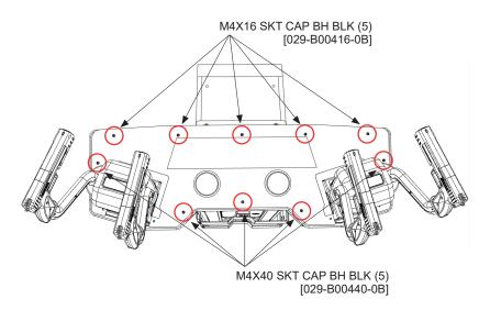
Open the COIN DOOR and disconnect the BUTTON HARNESS. Carefully remove the CONTROL PANEL COVER.
