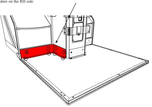
Secure the (4) M6 fixings on the **Bracket Floor Locating Mid (MI-9006XUK)**
