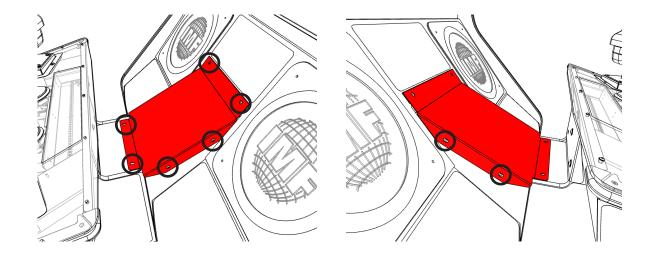
Secure the (8) M6 fixings on the **Bracket Floor Locating LH (HDZ-9003XUK)** and perform the same procedure on the RH side
