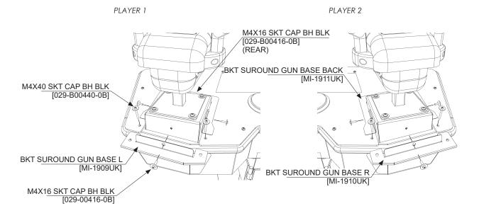
Remove the (5) M4X40 SKT CAP BH FLK fixings from the lower section of the CONTROL PANEL COVER and (5) M4X16 SKT CAP BH BLK fixings from the upper section.
