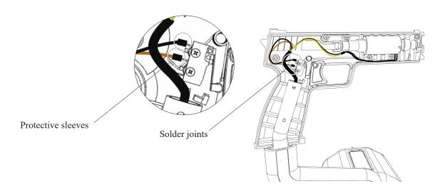
Replace the switch and re solder the wires onto the new switch in their correct locations. Ensure that the protective sleeves are also replaced
