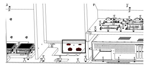
Secure the (8) M6X30 fixings on the Bracket Cover Joint Ctrl Cabi (MI-7059XUK)
