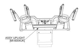
**7** Disconnect the ASSY UPLIGHT, remove the Cable Ties which secure the ASSY UPLIGHT into position. Remove the ASSY UPLIGHT.
