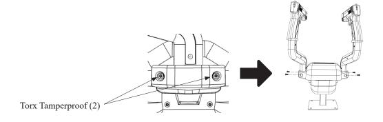
Remove the (4) Torx tamperproof fixings from both sides of the controller to remove the center cover
