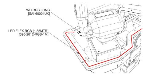
Replace the LED FLEX RGB [390-2012-RGB-1M] at a length of 1.85M. Reconnect the ASSY LED CLIP and assemble following these instructions in reverse order.
