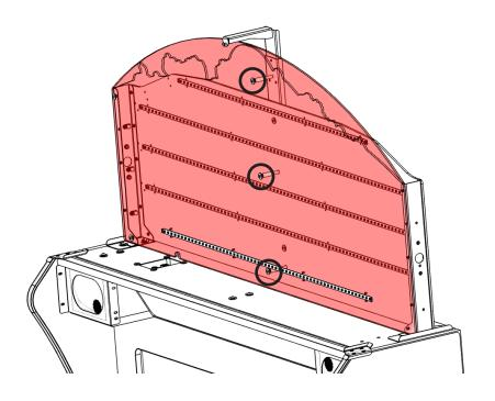
Insert **Strutt Sup Header Front (MI-5701XUK)** into positon on the right hand side and apply the (2) M6 highlighted fixings
