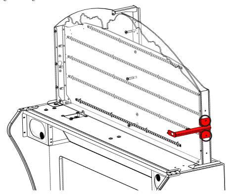
Insert the Bracket Cross Supp Header Mid (MI-5702XUK) and secure using the (2) M4 highlighted fixings
