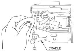
After wiping off as per previous step, further apply a dry cloth to completely dry the Coin Selector.
