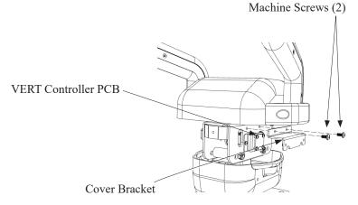
Remove the (2) machine screws which secure the VERT controller PCB bracket. Then remove the (4) machine screws which secure the PCB to the bracket. Carefully remove the PCB
