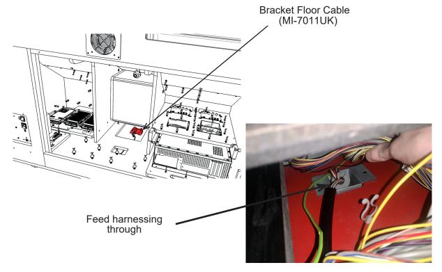
Connect the Harnesses from the Monitor Cab to the Coin Tower
